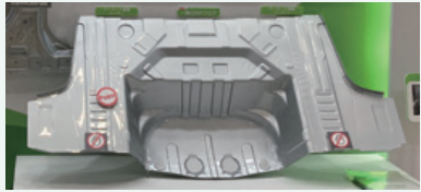
Deep-drawn rear floor pan integrating six parts by tailored welding
