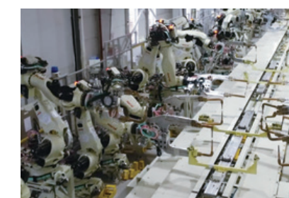
Assembly and welding equipment
